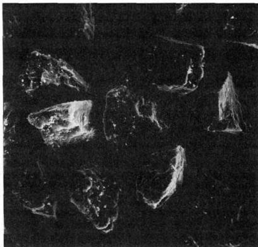
Figure 2.27 Scanning electron microscope photograph of pulverized coal particles.
